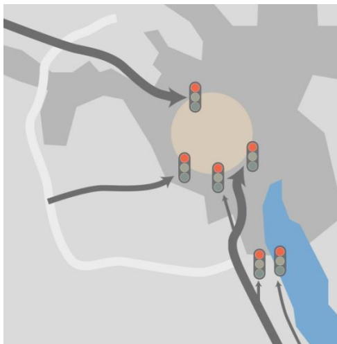
Traffic lights at the city borders to control the flow into town - automatic adaption according to the traffic volume with sensors in streets
