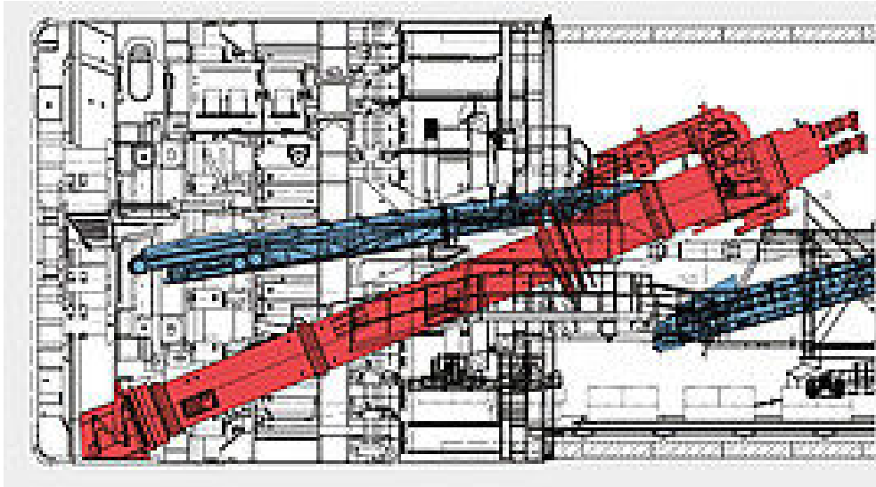
Figure 30 : Example of a multi-mode TBM (change open mode / EPB mode, www.herrenknecht.com )
