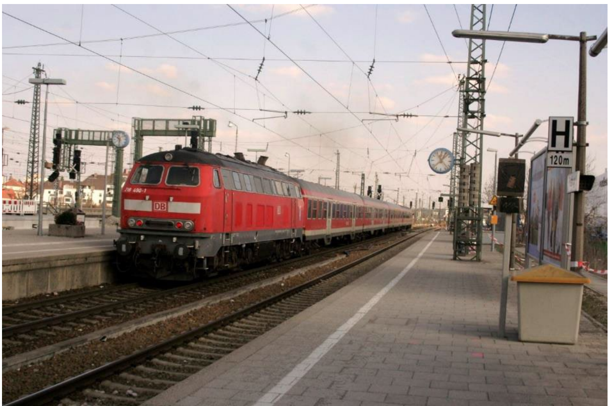
Figure 17. Diesel loco 218490 on the rear of a push-pull single-deck trainset at München Pasing
