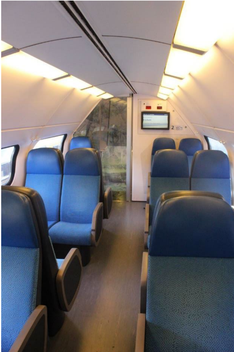
Figure 4. Upstairs Interior of NS double-deck EMU 9575, Netherlands Note restriction on height imposed by the loading gauge
