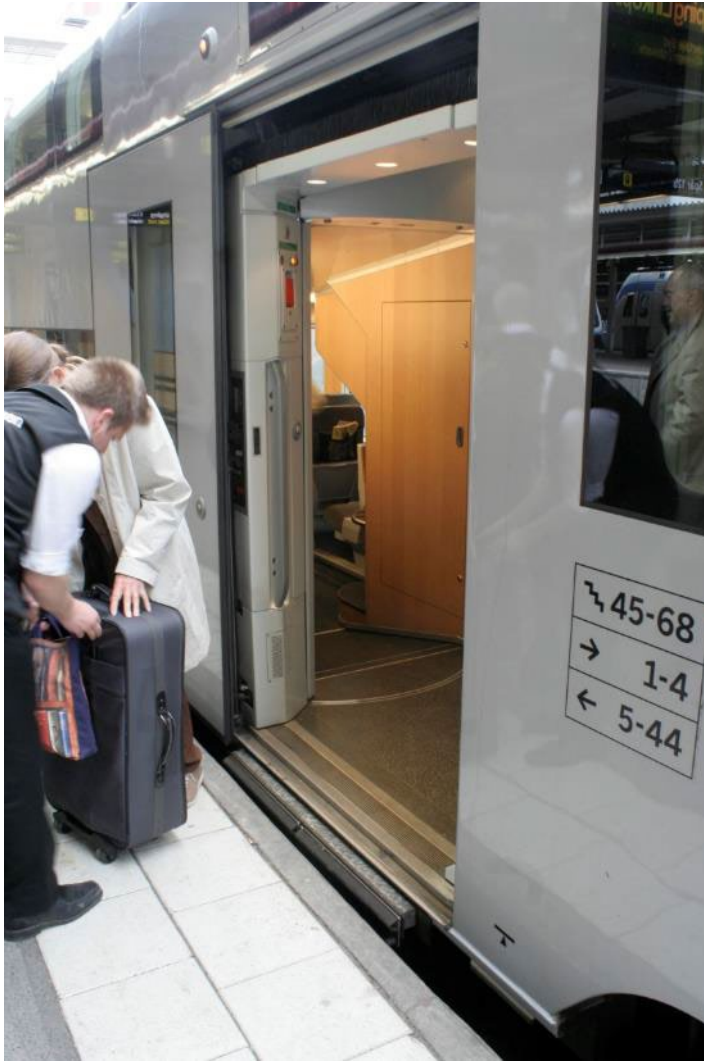
Figure 5. Ramp into lower level of SJ double-deck EMU 3333, Sweden
