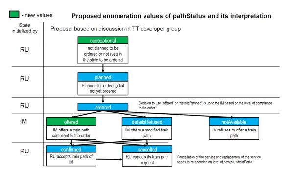
Figur 4: Process flow for @pathStatus (source: iRFP)
