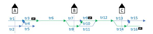
Figure 1: Microscopic track model of 3 stations
